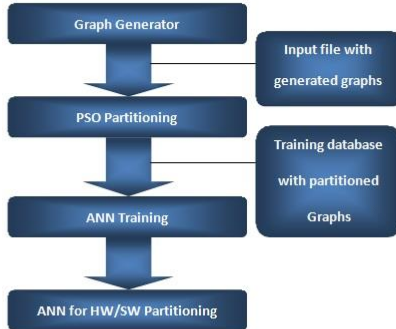
Figure 3. Proposed method's steps. Initially graphs are generated using precisely described technique. After the generation a PSO algorithm partitions generated graphs. After the partitioning a database is created with each generated graph and their respective partitioning as input/output pairs.
